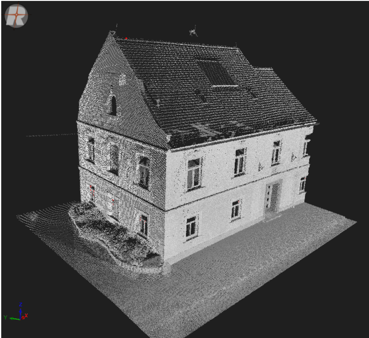
Figure 8: Point cloud data from a building in a village from two drive-bys, four scan data combined. Brightness gives reflectivity of surface in the range -25 dB to +5dB.
