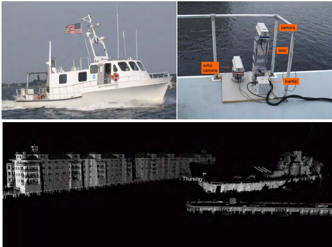
Figure 2.33: The vessel based mobile mapping system Bay-Hydrographer (Top left), the mounting bracket and mapping sensors (Top right) and first survey results of the battleship Wisconsin (Bottom) (VAN RENS et al., 2010)
