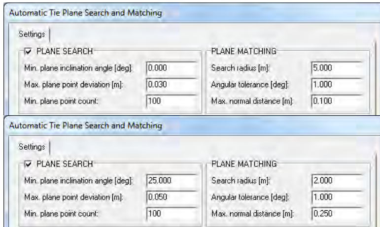
Figure 4.15: Plane search and matching parameters for scan data adjustment. (Top) Default values for mobile mapping; (Bottom) User defined
