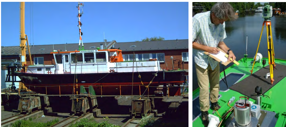
Figure 3.13: Initial measurement procedure to determine the lever arms off all integrated sensors with respect to the vessel's reference frame; Deepenschriewer III on a slipway in former times (Left); Lever arm measurement in water (Right)
