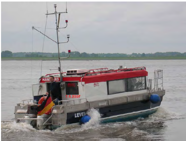
Figure 3.2: Survey boat "Level A" of the NIAH during a survey. As a standard sensor a RESON Seabat 8101 multibeam echosounder is bow-mounted
