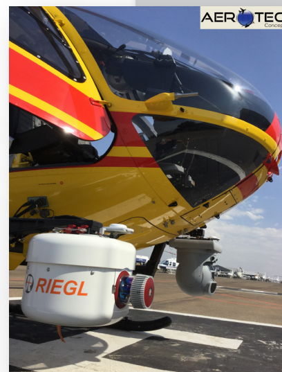
mounting example on a helicopter (EC135) for power line mapping/inspection
