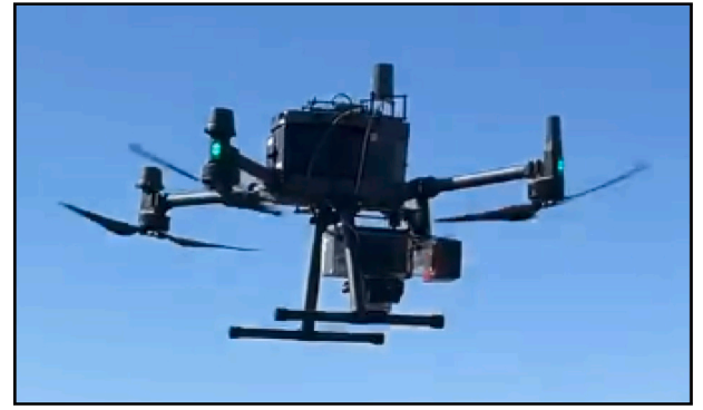
Fig. 7. DJI M350 with a RIEGL miniVUX-3UAV laser scanner and integrated RiLOC-E navigation system.
