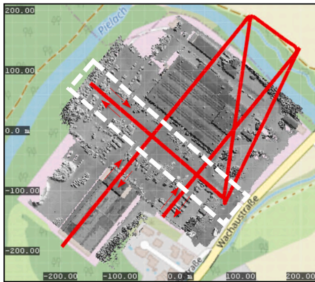
Fig. 8. ULS point cloud colored by reflectance (dark/bright = low/high reflectance, hillshade) and flight trajectory, superimposed onto map (© OpenStreetMap contributors). The X/Y-axes are those of a local east/north/up (ENU) Cartesian coordinate system. The point clouds from the two flight strips in the dashed white rectangle are later evaluated in detail.
