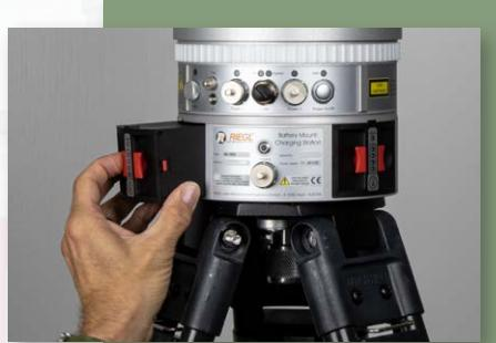
battery packs can be changed individually while scanner in use
