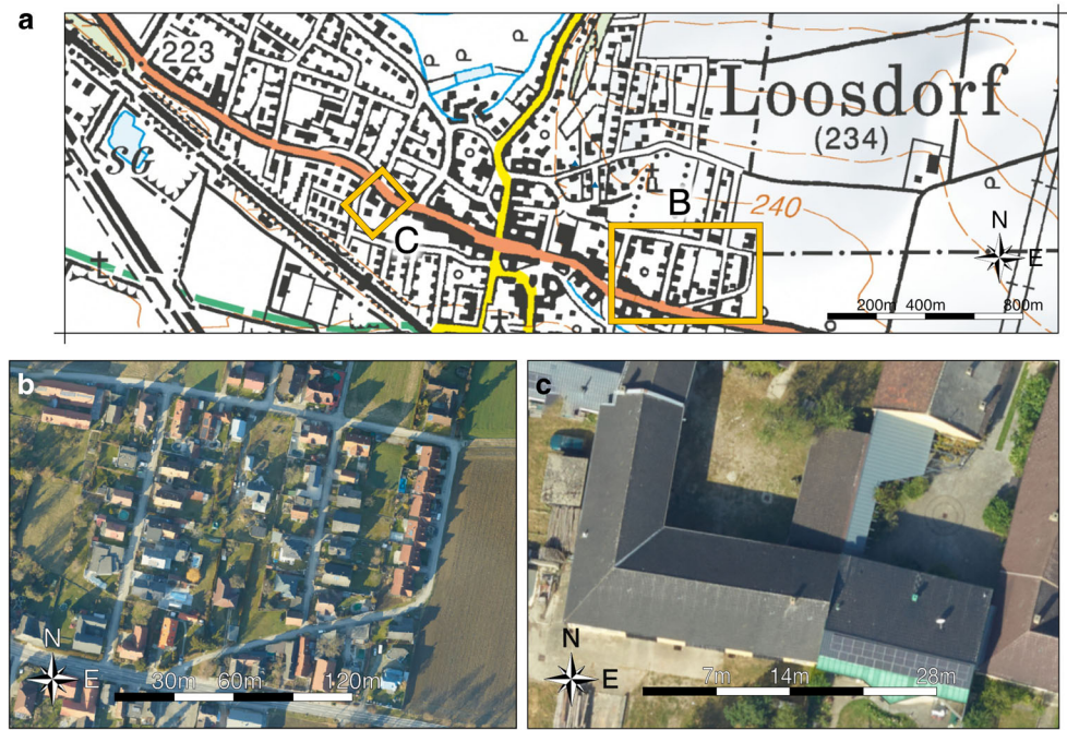
Fig. 3 a Map of the study area in Loosdorf, Lower Austria (Bundesamt für Eich- und Vermessungswesen 2024), where the first dataset ( b ) is marked with B and the second ( c ) with C. In contrast to the first dataset ( b ), which only consists of airborne LiDAR data, the second dataset ( c ) was surveyed with both airborne and terrestrial LiDAR; the latter as an additional reference.
