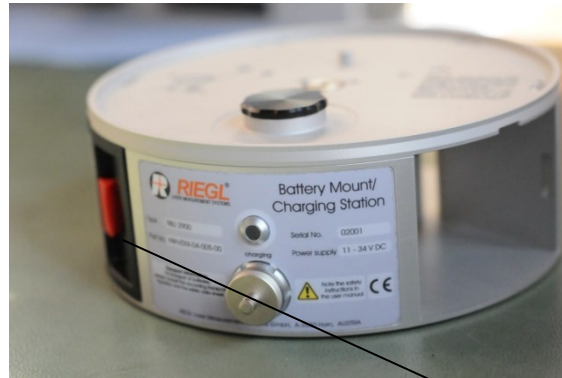
Fig. 18 Battery Mount / Charging Station RBLI 2900 with only one battery pack AP-RBLI 2903 inside
