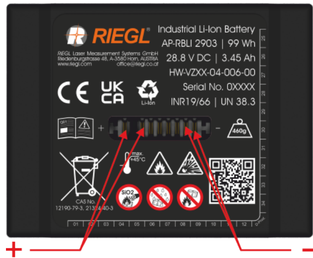
Fig. 4 Position of the poles, plus and minus pole, two pins each
