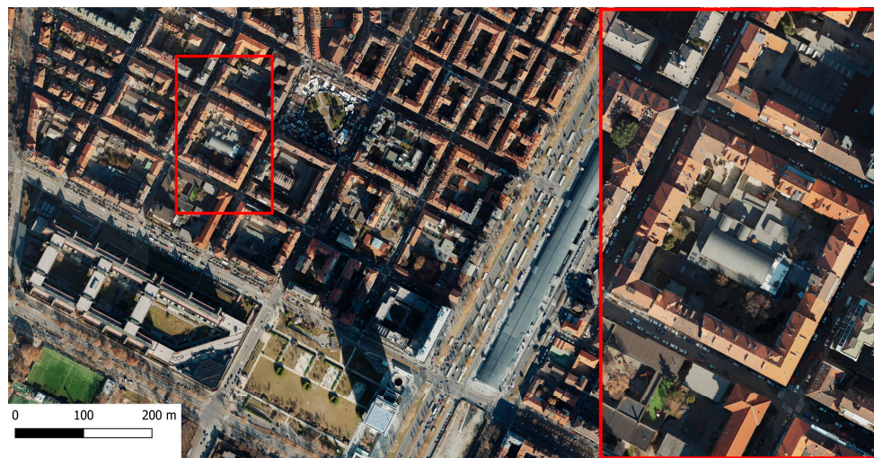
Figure 3. An orthophoto (dated February 2022, flight altitude 1000 m) illustrates, with a magnified area, the urban environment with dense shading caused by very close buildings and narrow streets.
