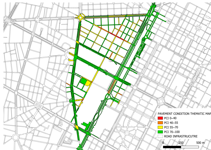
Figure 13. This map categorizes road segments based on their assessed condition, ranging from 0 to 100, where 100 represent the best condition, allowing for the data-driven prioritization of maintenance activities.
