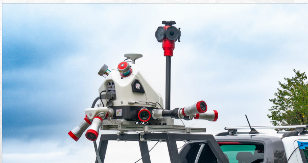
RIEGL VMX-2HA with 6 horizontally aligned RIEGL cameras (6 x 24 MP), the RIEGL pavement camera system (2 x 12 MP) as well as a 72 MP Ladybug 6 spherical camera system
