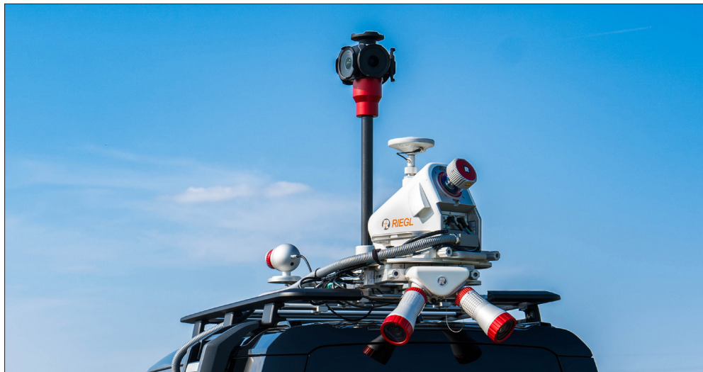
RIEGL VMQ-1HA with Ladybug 6 and Pavement Mount for two RIEGL tube-shaped cameras; two special mounting adapters at the front are ready to also carry these cameras for landscape data acquisition
