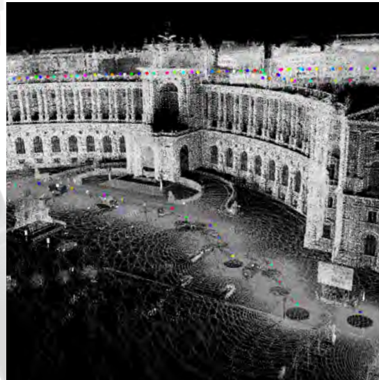
scan data detail, reflectance-scaled
