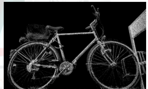
data after elimination of the „invalid“ points
