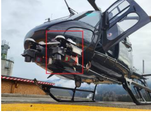
Figure 5. Helicopter platform with RIEGL VUX-160 23 laser scanner and RiLOC-E 25 IMU/GNSS navigation system, operated by Alto Drones . The second laser scanner is not used.
