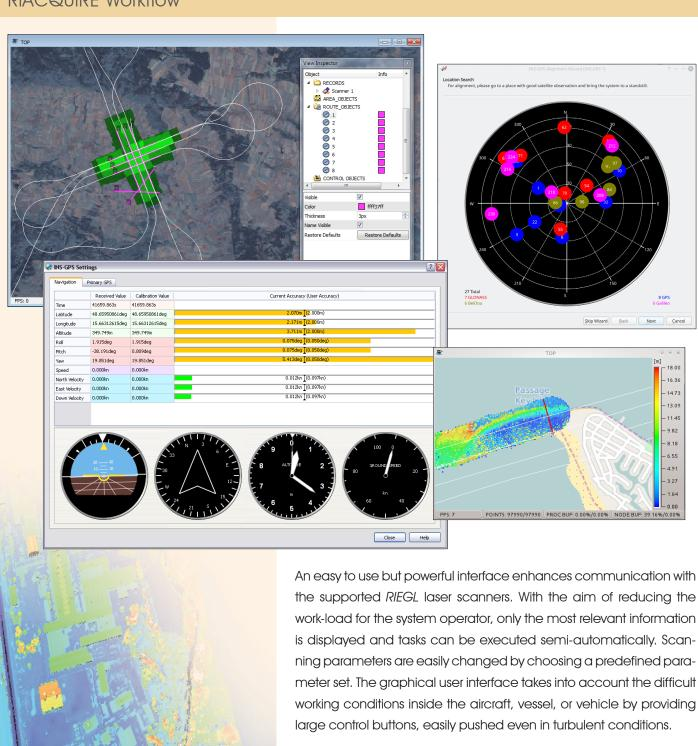
the supported RIEGL laser scanners. With the aim of reducing the work-load for the system operator, only the most relevant information is displayed and tasks can be executed semi-automatically. Scanning parameters are easily changed by choosing a predefined parameter set. The graphical user interface takes into account the difficult working conditions inside the aircraft, vessel, or vehicle by providing
