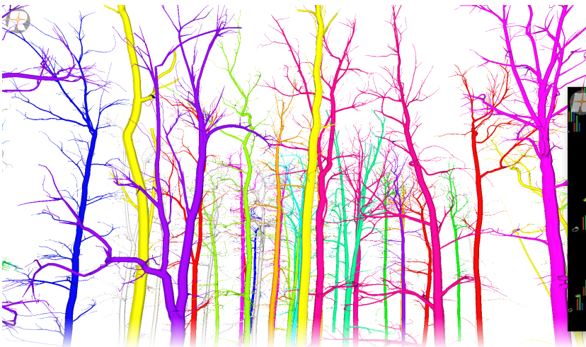
Segmented trees colored according to a unique tree ID: Each tree is georeferenced. A so-called pipe model is created for each tree – this is used to perform a highly accurate volume calculation. Branches can also be separated from trunks.
