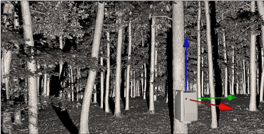
Single scan in forest environment: RIEGL VZ-600i, point spacing 6mm@10m, 25 sec scan time, pictures included
