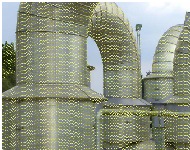
Fig. 2: Visualization of laser-scanner and photogrammetric data in superimposition
