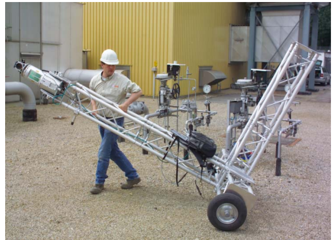
Fig. 14: Shifting the scanner by a mobile rack
