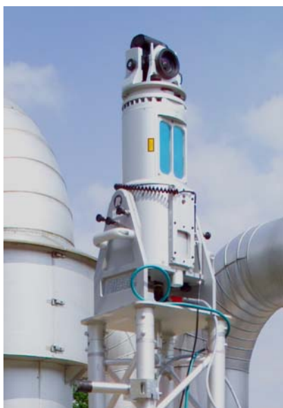
Fig. 1: Riegl scanner LMS-Z420i with mounted camera Nikon D100
