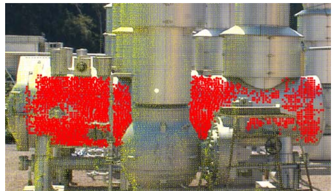
Fig. 7: Automatically aggregated points of cylinder surface
