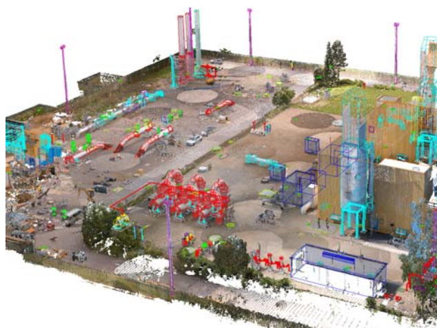
Fig. 20: Visualization of the dyed 3D-pointcloud together with the modeled elements
