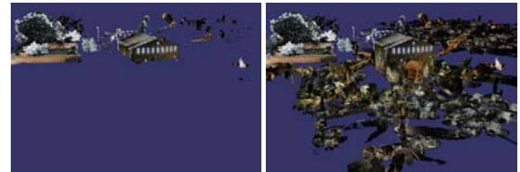
Figure 8: The basilica is partly above and partly below ground level. (Left) The point cloud is cut at the ground level, so that only objects above ground remain visible. (Right) Showing the whole catacomb, including the subterranean areas, the enormous expansion of the catacomb underground becomes visible.
