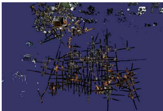
Figure 1: The model of the Domitilla Catacomb from bird's eye view. The model consists of 1.2 Billion points.
