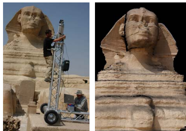
Fig. 6: Top: High resolution scan from the Sphinx from a distance of 570 m from the top of the Cheops Pyramid visualised as point cloud. Bottom: Left: Scanner mobile in front of the Sphinx. Right: Triangulated point cloud of a single scan textured with the digital image.
