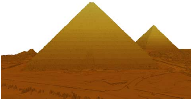
Fig. 3: 3D visualisations of the triangulated point cloud measured from the top of the Cheops Pyramid using ARC GIS 8.2.
