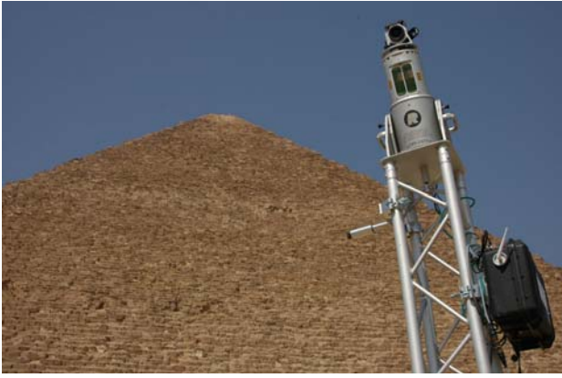
Fig. 1: RIEGL LMS-Z420i Laser Scanner with a calibrated high resolution digital camera Nikon D100, both connected to a WLAN-box in front of the Cheops pyramid.
