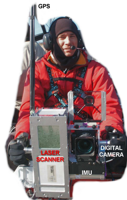
Figure 2: The handheld block composed of all the devices: digital camera, laser scanner, GPS antenna and IMU.
