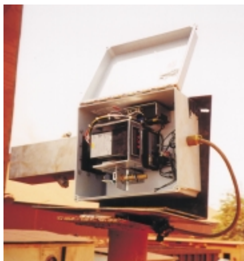
LD90-450 in industrial enclosure (open) with lens protection tube
