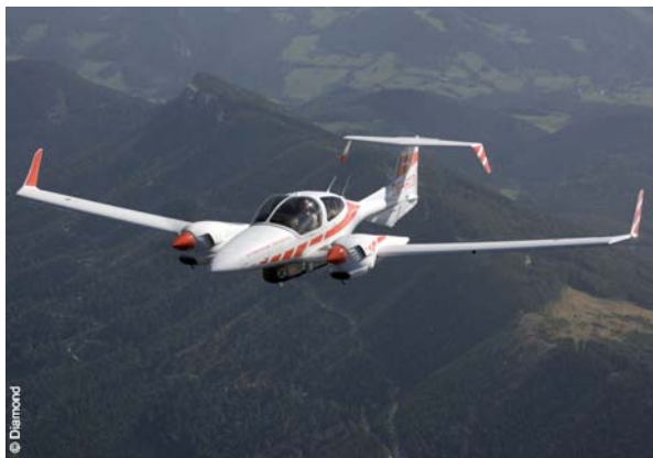
The Diamond Aircraft multi purpose platform fleet: DA42-MPP and HK36-MPP each equipped with RIEGL airborne laser scanners LMS-Q560
