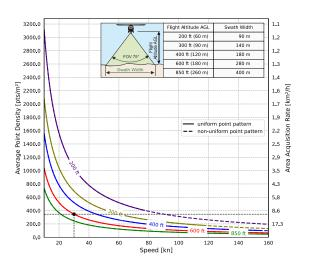
Example: VUX-180 $^{24}$  at 1,800,000 pulses/sec, laser power level 100% altitude 600 ft AGL, speed 30 kn, resulting point density  $\sim 346.3$  pts/m $^2$
