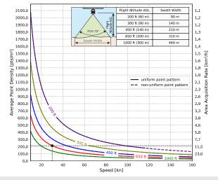
Example: VUX-180 $^{24}$  at 1,200,000 pulses/sec, laser power level 100% altitude 650 ft AGL, speed 30 kn, resulting point density  $\sim$  213.1 pts/m $^2$
