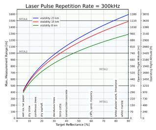
Operating Flight Altitude AGL given for the following conditions: FOV 75°, ambiguity resolved by multiple-time-around (MTA) processing, average ambient brightness, target size ≥ laser footprint, roll angle <±5 deg
