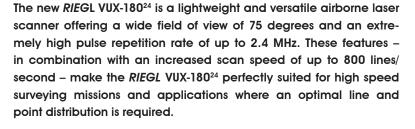
The RIEGL VUX- $180^{24}$  makes use of RIEGL's unique Waveform-LiDAR technology, allowing echo digitization and online waveform processing. Multi-target resolution is the basis for penetrating even dense foliage.
