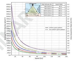
Example: VUX-180 $^{24}$  at 2,400,000 pulses/sec, laser power level 100% altitude 550 ft AGL, speed 30 kn, resulting point density  $\sim$  503.7 pts/m $^2$
