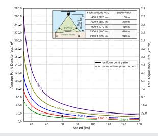
Example: VUX-180 $^{24}$  at 300,000 pulses/sec, laser power level 100% altitude 1,300 ft AGL, speed 60 kn, resulting point density  $\sim 13.3$  pts/m $^2$
