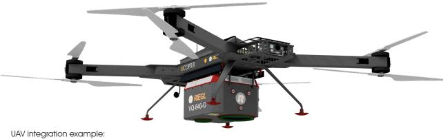
RIEGL VQ-840-G installed on RICOPTER-M
