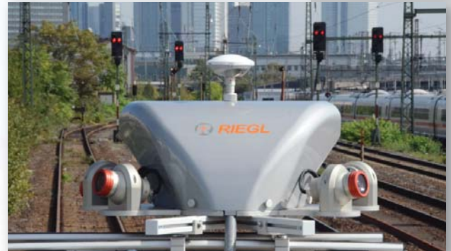
mounting frame interface to different railcars
