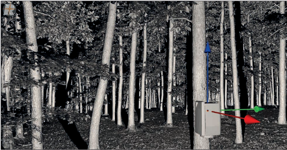
single scan in forest environment: RIEGL VZ-600i, point spacing 6mm@10m, 25 sec scan time, pictures included
