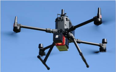
RIEGL miniVUX-SYS with Integration Kit 300 on DJI M300
