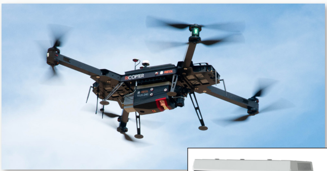
RICOPTER with RIEGL VUX-240 LiDAR Sensor, APX-20 UAV and nadir RGB camera
