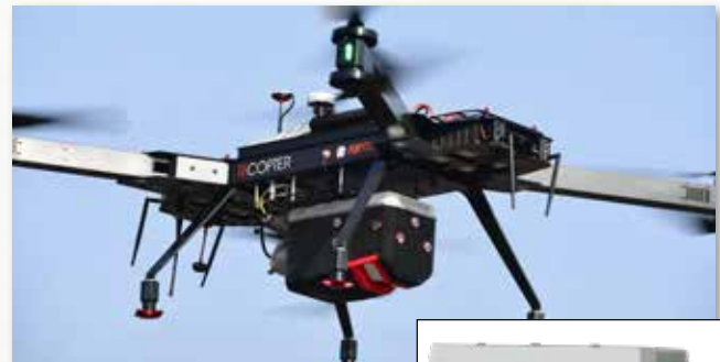
RiCOPTER with RIEGL VUX-240 LiDAR Sensor with APX-20 UAV fully integrated
