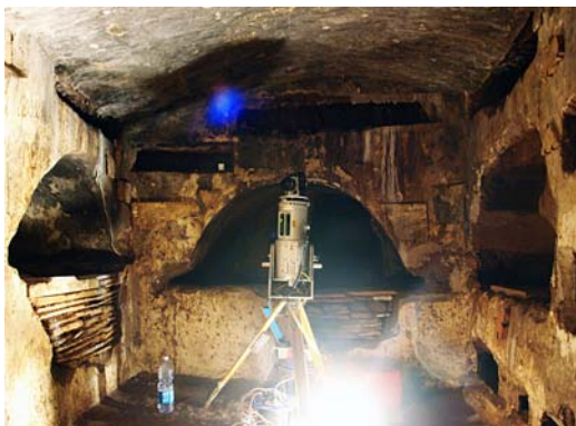
Fig. 6 – Laser scanner Riegl LMS Z420i on site
