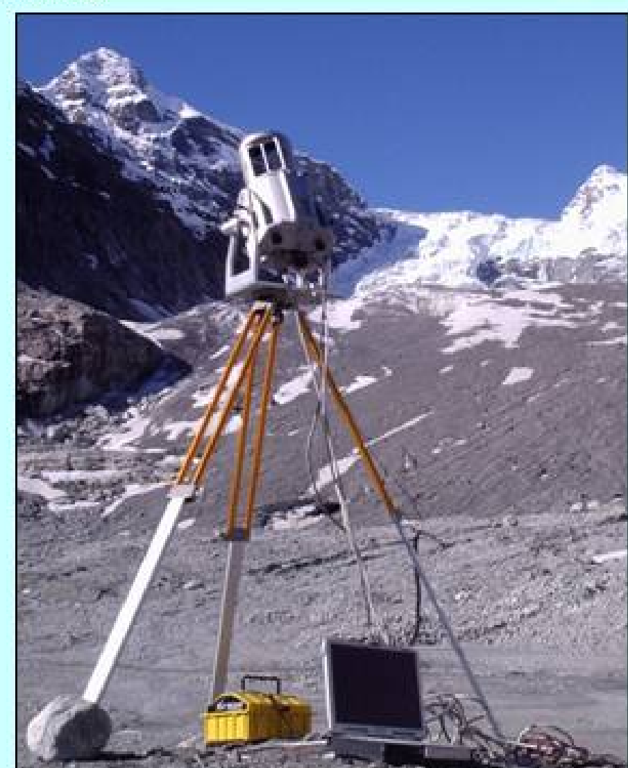
Fig 2 Riegl LMS Z210 side scanning laser.
