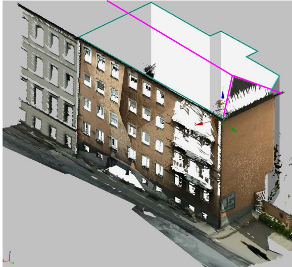
Figure 3-1. Building modelling from hybrid scandata.
