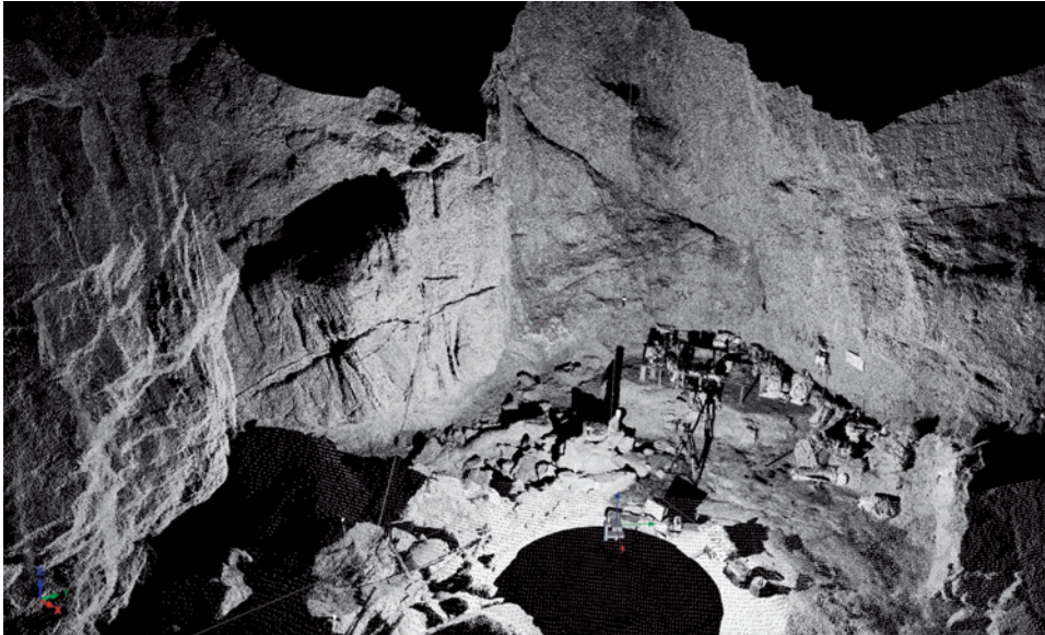
Fig. 5: Illustration of an \sim 200^\circ sector of the point cloud of one single rotational laser scan showing the rock pulpit (“plateau”) where (the former) Bivouac 1 is located below the rock face in the background (cf. Figs. 7–9). Note the rope of the suspension bridge (lower left) and another fixed rope obliquely leading some 25 m up the rock face to the cave tunnel which leads to the Schladming Shaft. Distance from viewing point to far range approx. 25 m.
