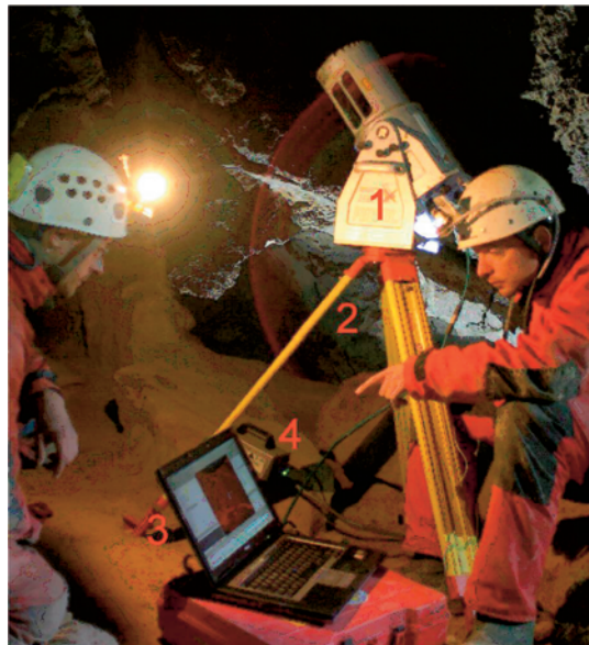
Fig. 4: Operating the Riegl LMS Z420i at a rock pulpit in the Ramsau Dome. Location cf. Fig. 2. For explanation of the figure see text above.
