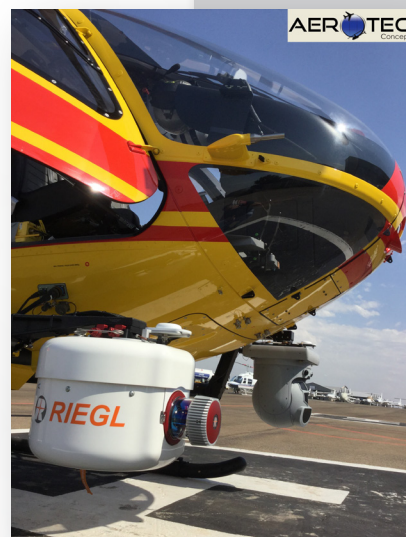
mounting example on a helicopter (EC135) for power line mapping/inspection
