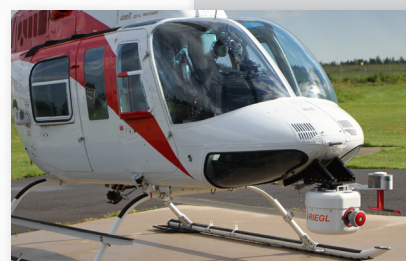
mounting example on BELL Long Range Helicopter
