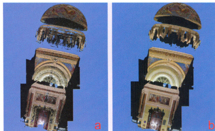
FIG. 4 A-B - Grazie's Church interiors: comparison between photo-texturing over a point model (a) and over a meshed model (b)
