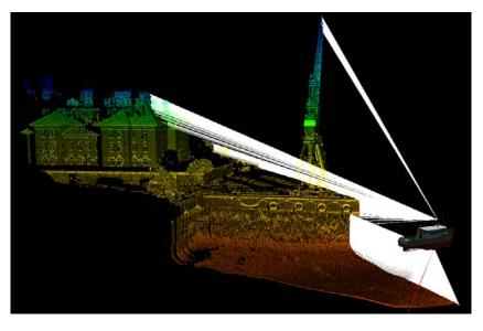
During data acquisition PDS2000 displays in real time the Laser data together with the Multibeam data in one 3D view. To control data quality for these large datasets the real-time 3Dvisualisation is a very strong QC tool. Other views are also available as per choice of the surveyor.
