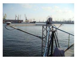
During an integrated Multibeam laser scanner project in the Port of Constanta, Romania, Shark SRL using their Riegl Laser scanner, a RESON SeaBat 7125 multibeam Sonar and an Applanix Wavemaster system providing attitude- and positioning information discovered that the PDS2000 was the perfect tool for Shark Survey to acquire and process the data from all these sensors.
