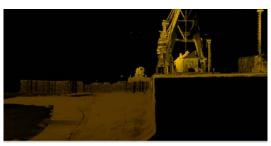
Both images show that when an accurate attitude and positioning system is used the multibeam and laser data match nicely.
