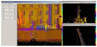
done by matching the point clouds of the different files (survey lines) with each other. The images below show an example of a non calibrated image. The masts on the building are a good point of focus same as the top of the cranes. On the main building the 3 bushes must be one as well. The correction is a combination of pitch and yaw.
