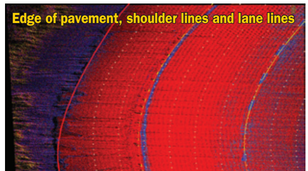
Figures 5-9. Extraction requirements for the project included standard topography break-line elements.
