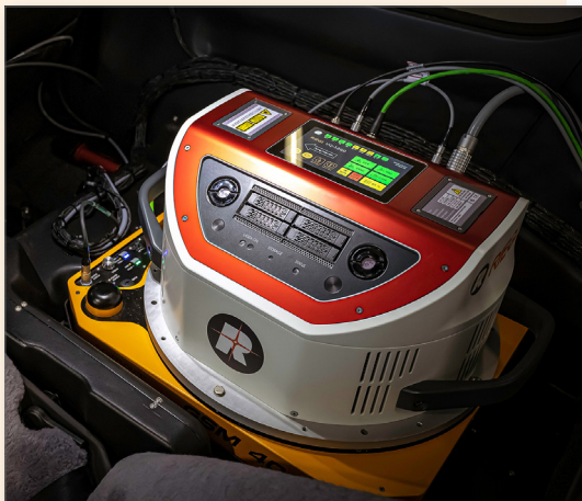
RIEGL VQ-1260 installed on the GSM-5000 gyro-stabilized platform
