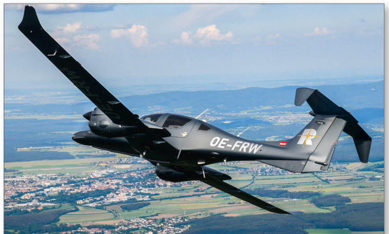
RIEGL VQ-1260 installed in the fuselage hatch of the Diamond Aircraft DA62 Survey Star
