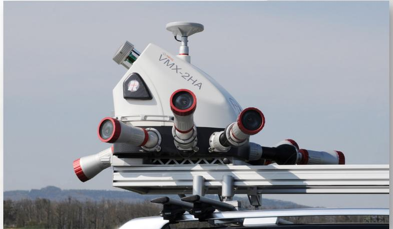
VMX-2HA equipped with 7 ball-joint directional RIEGL cameras
