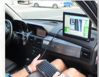
The VMX-2CU (equipped with a high performance 7th generation Intel Core i7 processor) precisely controls management of power, data acquisition, and operation of the laser scanners, INS/GNSS sensors and the optional cameras.
