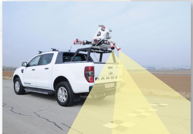
VMX-2HA equipped with 6 ball-joint directional RIEGL cameras, two ball-joint pavement cameras with close to NADIR orientation
